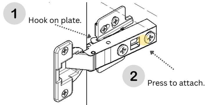
**3** A 'SNAP' sound is the confirmation of a successful installation.
