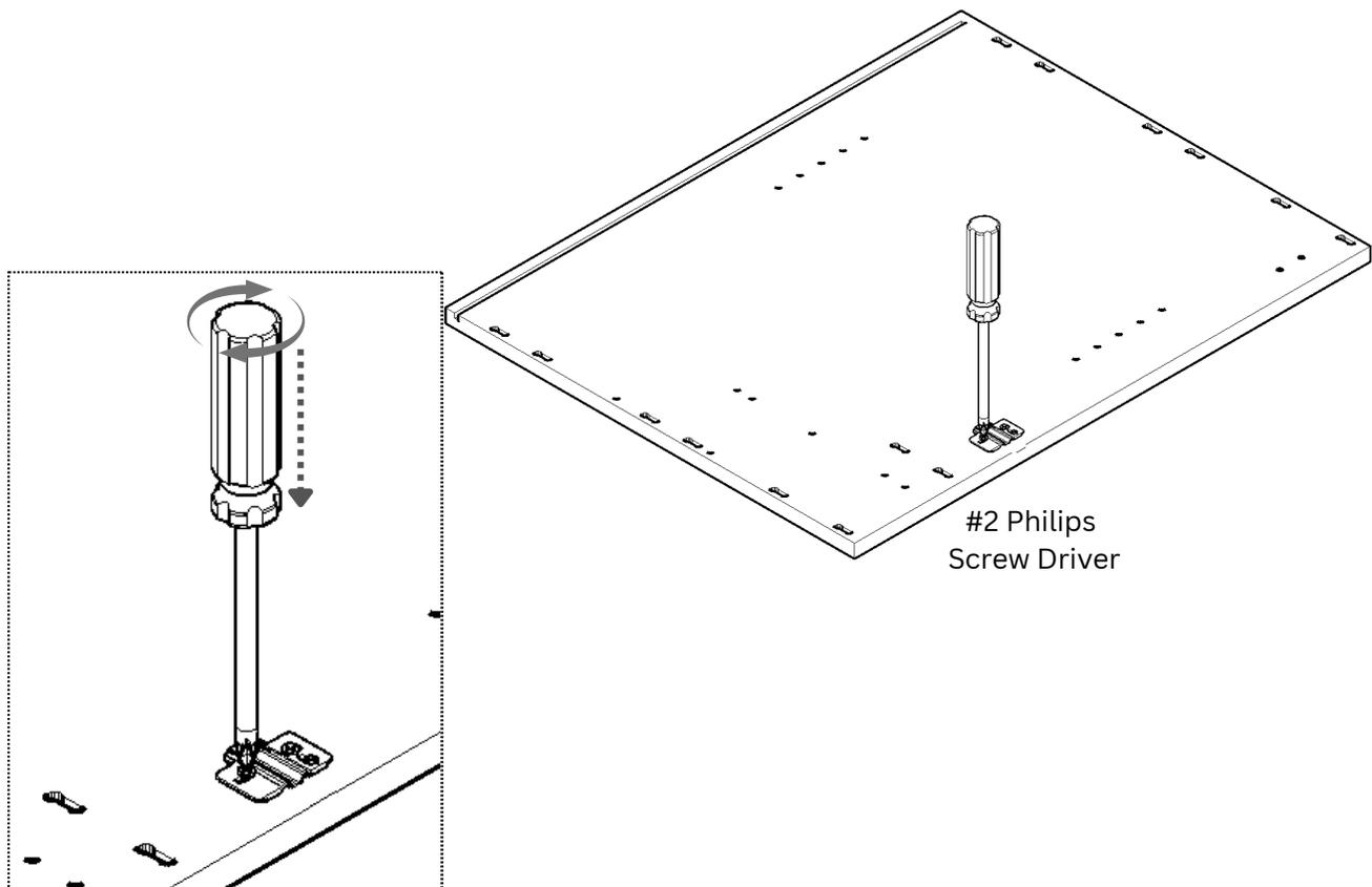
Take out the drawer glide and place it with the screw-hole side facing down
