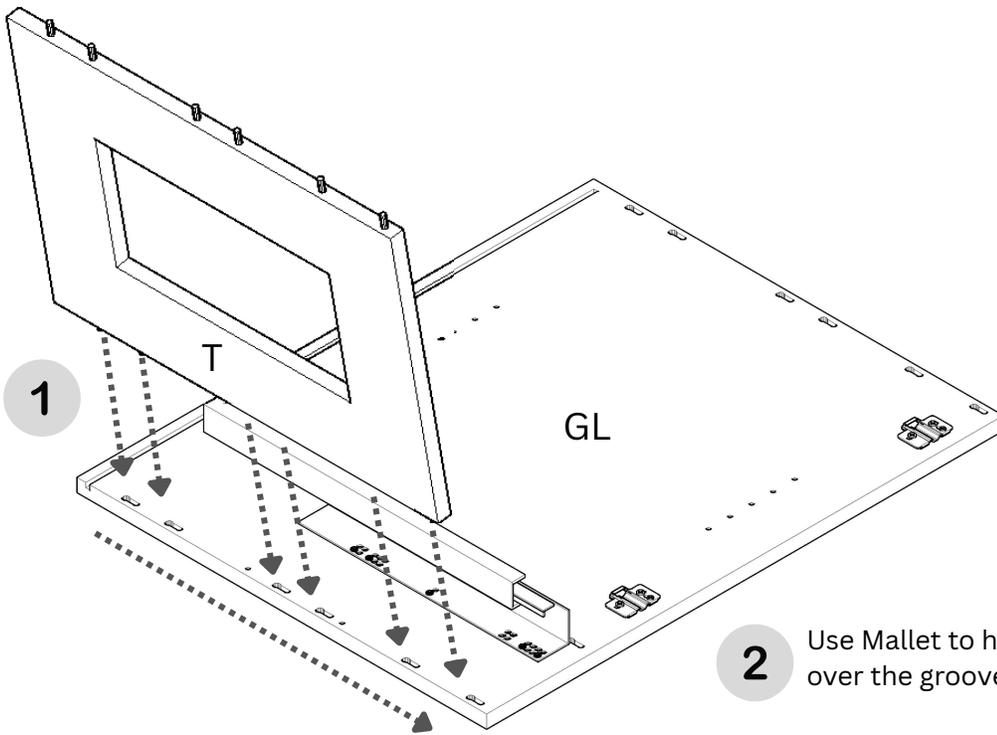
2 Use Mallet to hit the top panel all the way over the groove
